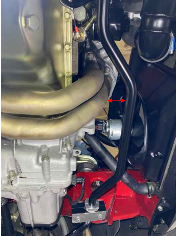
Optimized design for more space between sway bar and downpipe.
